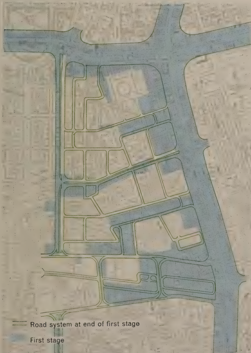
200 The roads as they would be at the end of the first stage. Where the roads fall outside the blue tint it indicates that use is made of existing streets.
